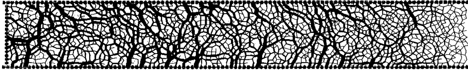
FIG. 9. Snapshot of the contact force network. The lines joining the centers of the particles in contact have a width proportional to the normal contact force.
